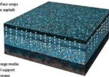
Figure 2.5: Three-Dimensional View of Permeable Pavement
